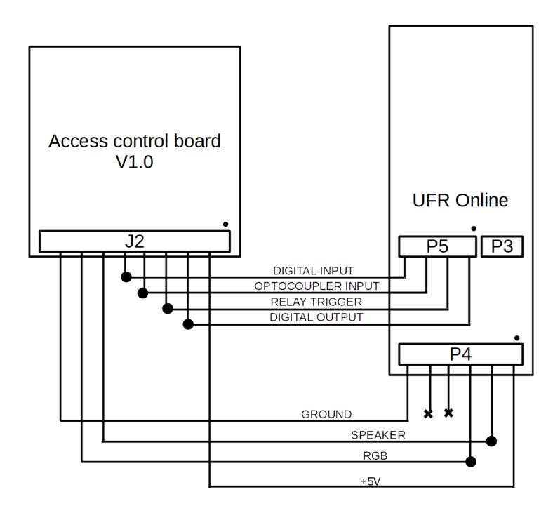
There is also a premade cable for connecting uFR Online and Access control board.
