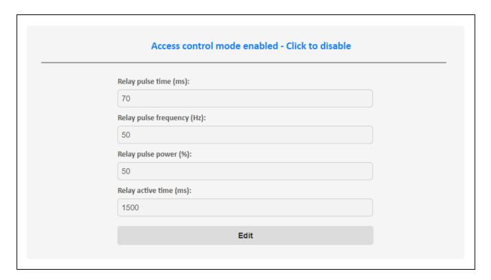
\*\*\*Access control mode must be enabled before the access control board is connected.
