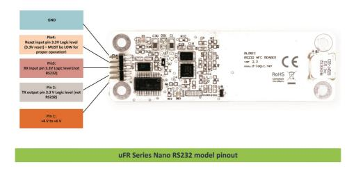
For communication purposes between reader devices and host PC, D-Logic's proprietary protocol called "uFR serial" is created.
