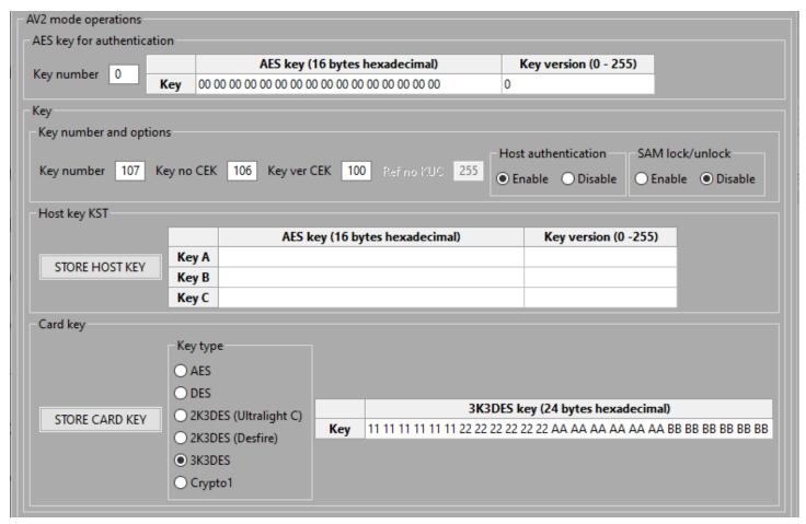
Card key parameters and values: Key no = 107, current Key no CEK = 0, current Key ver CEK = 0 (first key changing with master key A), futured Key no CEK = 106, futured Key ver CEK = 100 (Key A of KST 106), type of card key is 3K3DES (24 bytes), value of key 11 11 11 11 11 11 22 22 22 22 22 22 AA AA AA AA AA BB BB BB BB BB.
