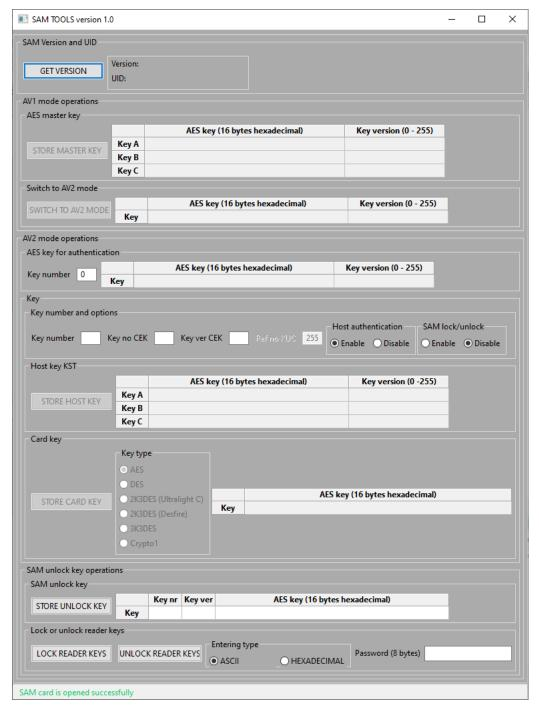
For proper functionality it is need connect the uFR Classic CS with SAM card to the PC. Firmware versions there support SAM are 5.100.xxx. For same hardware exist firmware versions 5.0.xxx, which does not support SAM, instead they uses keys stored into reader.
