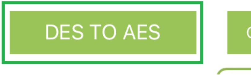
By using the provided **DES TO AES** button, the user will switch the card master key from the default DES key to the AES key.
